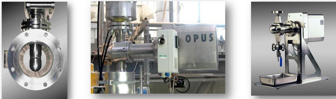
Fig. 4: UE probe OPUS in an in-line (left), in-line with by-pass adapter (centre) and off-line application. The devices cover applications with suspensions and emulsions in the range of 0.01 to 3000 mm, 0 to 70 %vol. without dilution, 0 to 40 bars, 0 to 120°C, pH 1 to 14, with GMP and ATEX versions as an option
