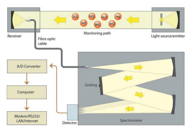
The basis of the principle used by OPSIS to identify and measure concentrations of different gases is scientifically well established: Differential Optical Absorption Spectroscopy (DOAS), which is based on Beer-Lambert's absorption law. It states the relationship between the quantity of light absorbed and the number of molecules in the lightpath.
