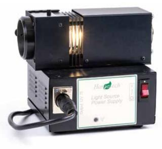
The lamp housing contains a cooling fan, infrared reducing "Hot-Mirror" and optics to provide light with minimum variation of intensity across the beam and little divergence from parallel. 2 slots are provided to accept 50mm square optical filters or a manual shutter plate.
