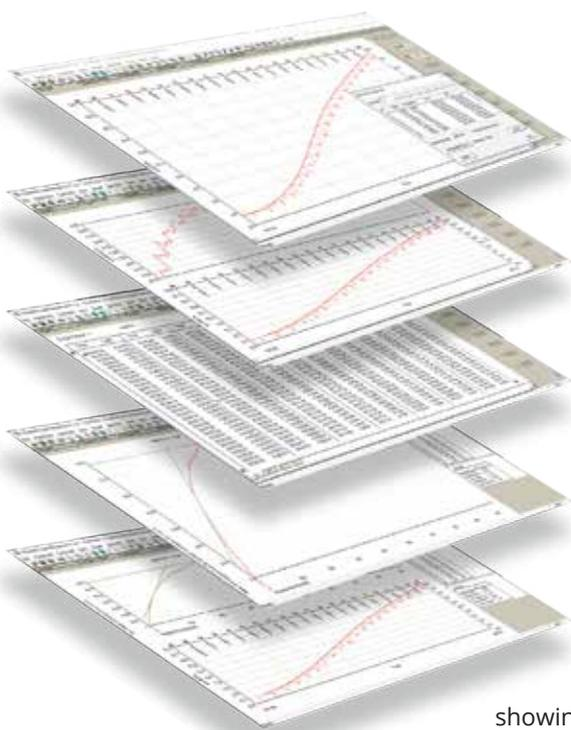
Post acquisition analysis tools allow automatic calculation of oxygen rates from user-defined rate intervals. Additional analysis tools automatically calculate rates of change for defined PFD light steps with a calculation of quantum yield presented at the end of a measurement. All files are saved as Comma Separated Values (CSV) data files opening effortlessly in external data processing packages such as MS Excel®.
